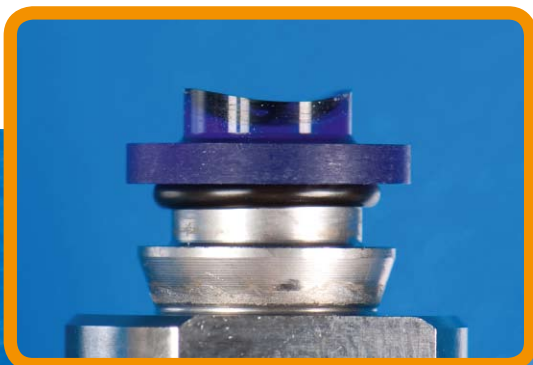
Contact lens blank with toric base curve
